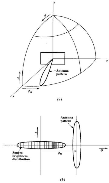
Fig. 3-3. Antenna pattern (a) and geometry for long source and fan-beam antenna pattern (b).
