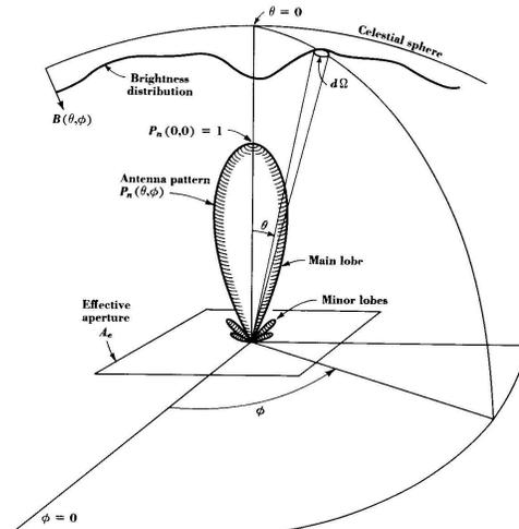
Fig. 3-2. Relation of antenna pattern to celestial sphere with associated coordinates.
