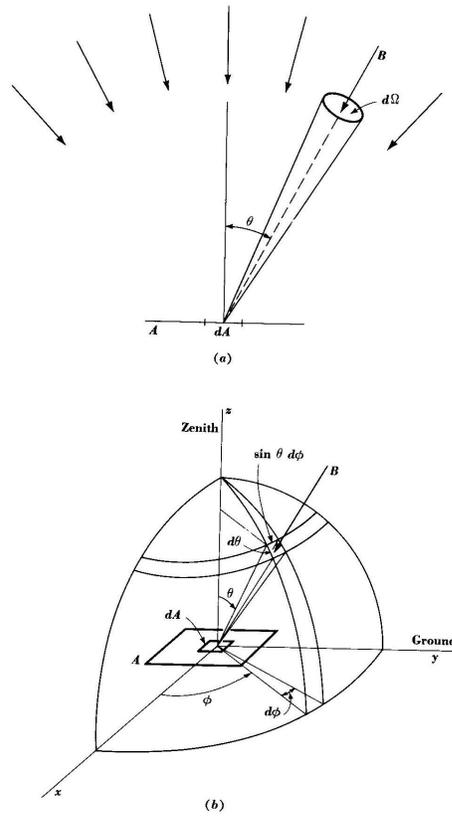
FIGURE 1. Basic geometry for radiation of brightness  $B$ , after [1, Fig. 3.1].
