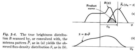
Fig. 3-4. The true brightness distribution  $B$  scanned by, or convolved with, the antenna pattern  $\tilde{P}$ , as in (a) yields the observed flux-density distribution  $S$ , as in (b).
