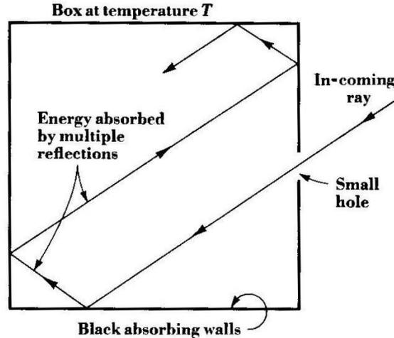
FIGURE 5. A blackbody enclosure, after [1, Fig. 3.11].
